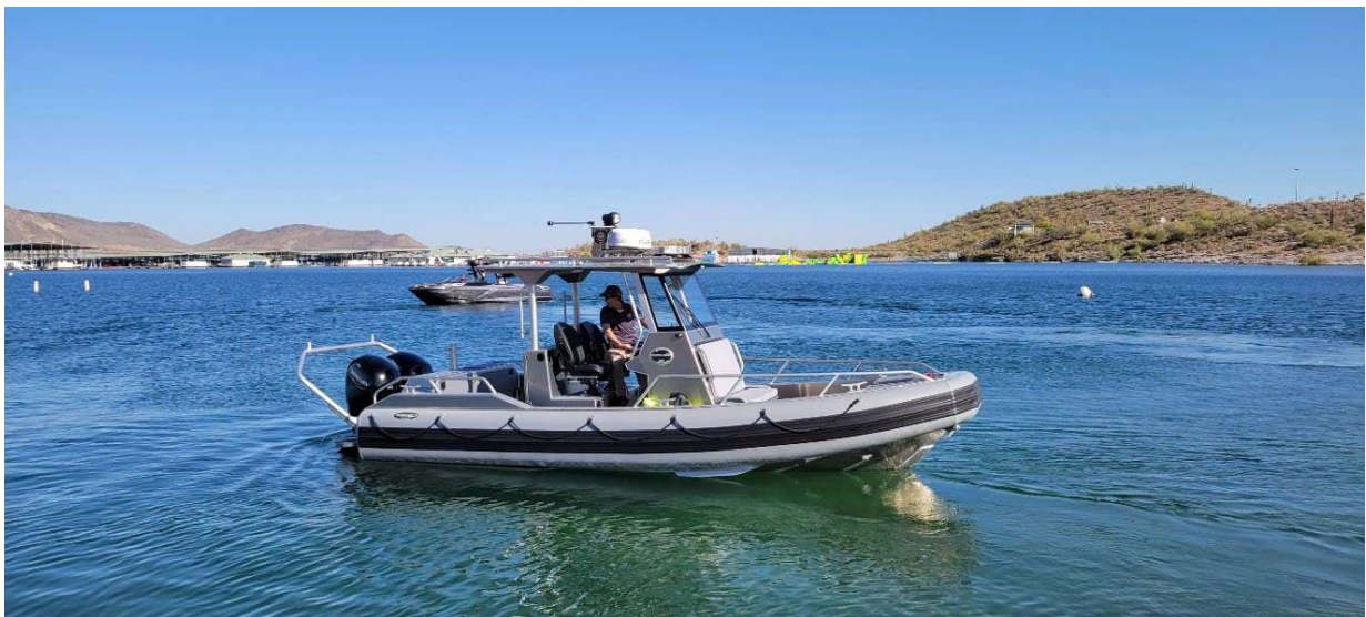
Photo 4: Modern RESCUE BOAT by Life Proof. Note the hard T-top solid roof with full windshield and built in wiper for protection from the elements and inclement weather.
