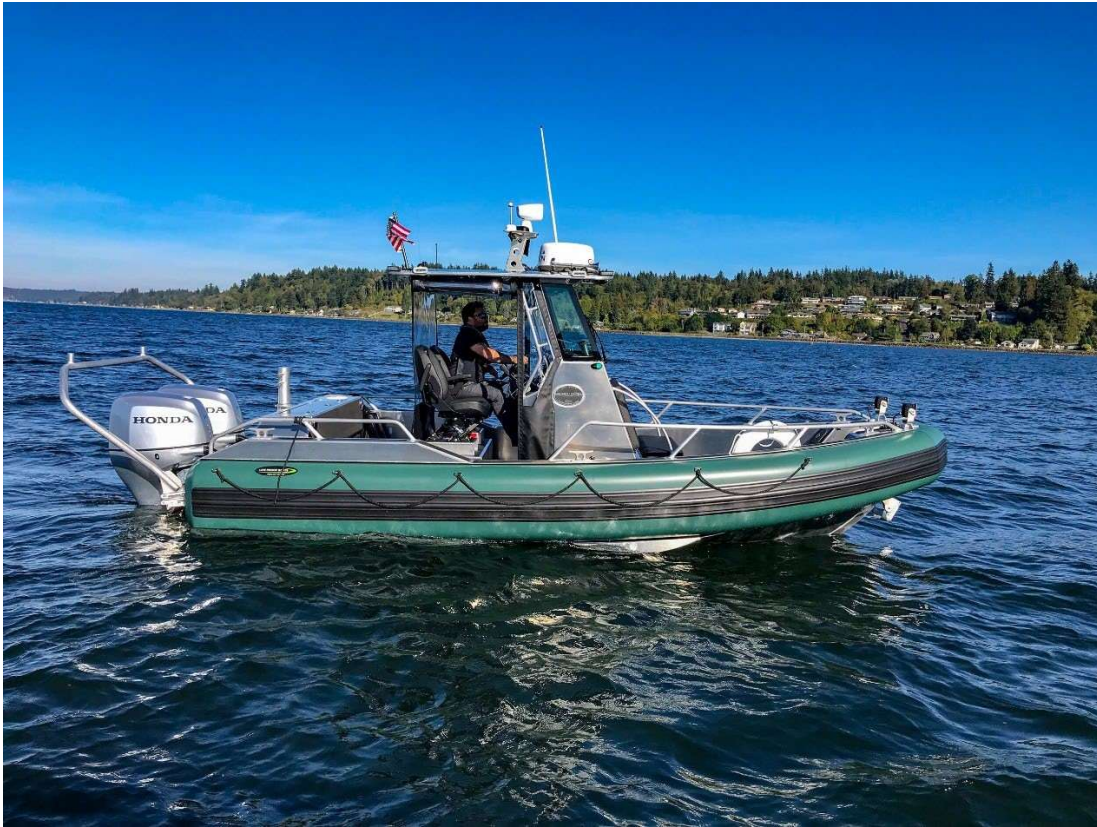
Photo 3: Modern RESCUE BOAT by Life Proof. Note the marine grade aluminum shell with the F.A.S.T. collar system. Foam Air Stabilized Technologies full collar wrap for safety & protection of the boat.
