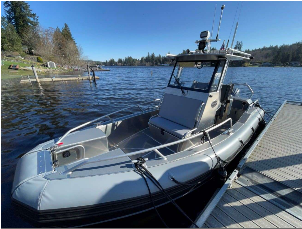
Photo 5: Modern RESCUE BOAT by Life Proof. Note the drop-down bow door with ladder and handrails. Also note the built in anchor system underneath the bow door.
